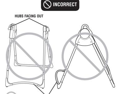
• Check to be sure you have assembled the leg assemblies to the bases correctly. Please refer to the illustrations above.
